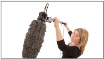
Boom microphones are sometimes covered in fur to reduce wind and environmental noise.
